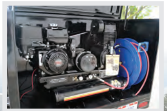
Air Compressor / Generator with 100' Air Hose Reel
